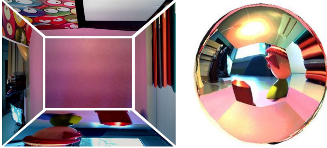
Fig. 7. Cubemap built with 6 HDR pictures (top view) and reflection on a sphere (front view).
