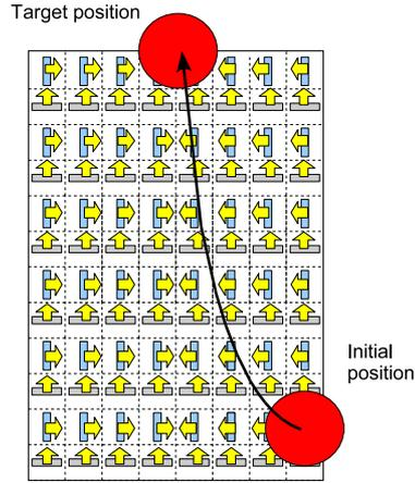
**Fig. 7** Vector field for the part-conveying task.
