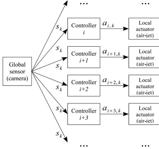
**Fig. 10** Semi-decentralized control architecture.
