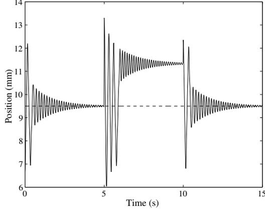
**Fig. 6** Position of the cylinder's center according to the time using programmable vector field (solid line), the dashed line represents the target position. Short perturbations are done at time steps 0, 5 and 10 s.
