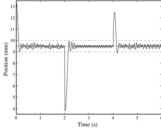
**Fig. 11** Position of the cylinder's center according to the time (solid line) after learning with the Q-Learning algorithm, the dashed line represents the target position. The control architecture is semi-decentralized. Short perturbations are done at time steps 0, 2 and 4 s.
