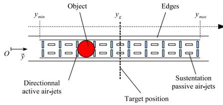
Fig. 4 Part-stabilization-task description.
