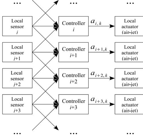
**Fig. 14** Fully-decentralized control architecture with sensors sharing.
