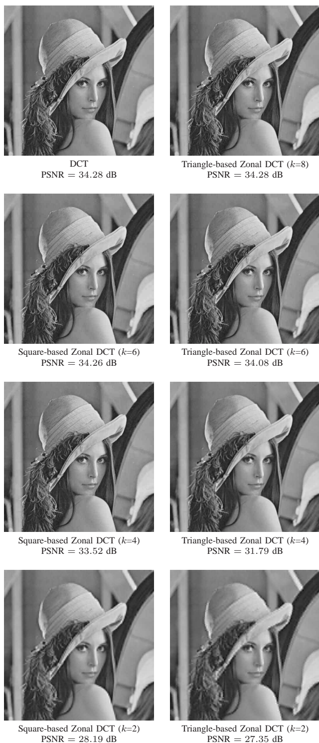
Fig. 4. Lena image coded at 0.5 bpp by regular DCT, Triangle-based and Square-based zonal DCT for different values of k .
