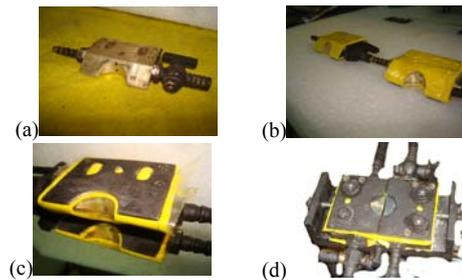
Figure 1 : Mounting the self-oscillating valve for the experiment: (a) bronze block with supply channels, (b) latex half mounted, (c) mounted latex on the two blocks, (d) endoscopic view of the mounted replica.
