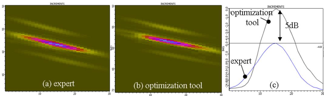
**FIGURE 3.** Imaging of the nozzle inspection. (a) B-Scan of the expert solution. (b) B-Scan of the optimization tool solution. (c) Comparison of echo-amplitude curve of solutions found by an expert and the optimization tool.
