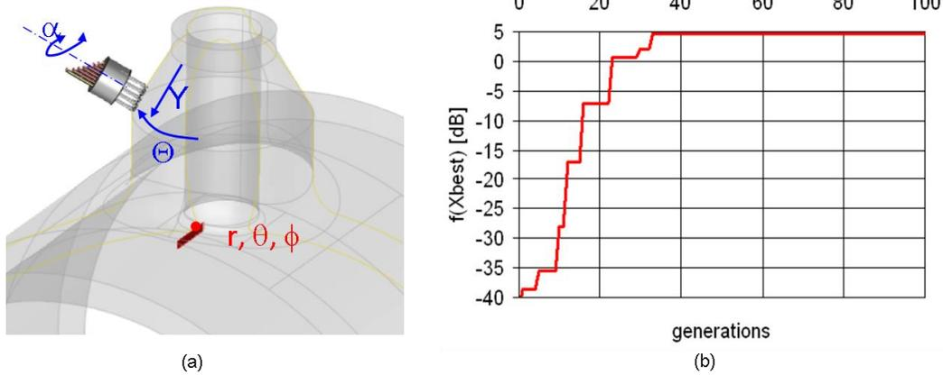
**FIGURE 2.** Optimization of a nozzle inspection. (a) Set-up of the inspection and definition of parameters involved for the optimization. (b) Evolution of the objective function of the best solution for each generation  $k = 0, \dots, 100$ . Values of the objective functions are given in dB compared to a solution found by an expert.
