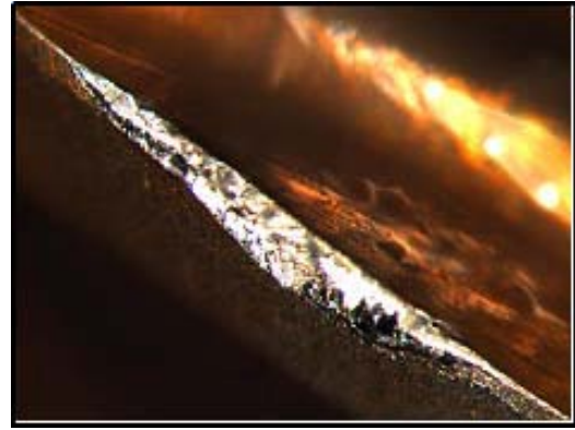
Fig. 5: Flank tool wear after 320 cuts
