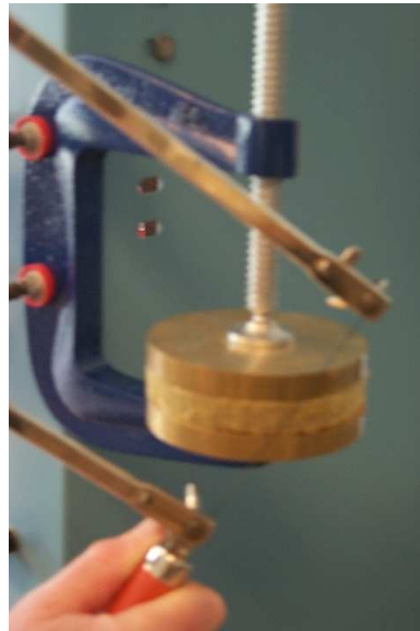
Figure 2.5: Carving system for large tool samples. The wire-saw used for this is seen at the foreground.
