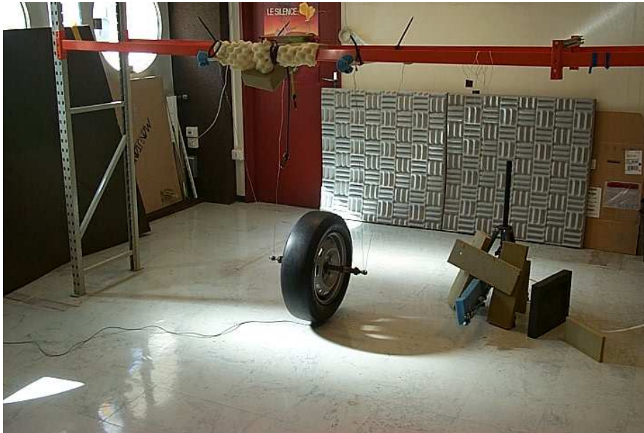
Figure 7.1: Global view of measurement for a single wheel over a rigid surface.
