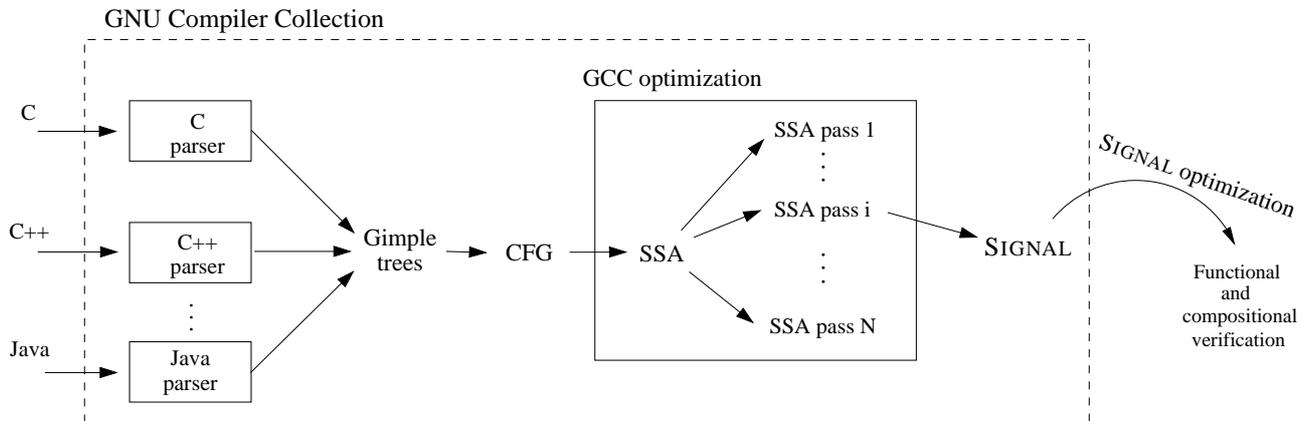
Figure 11. Translating C/C++ models into SIGNAL processes
