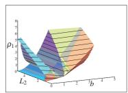
Fig. 5 The cells of  $\mathbb{R}^3$  where the manipulator admits cuspidal configurations, front view (left) and back view (right).
