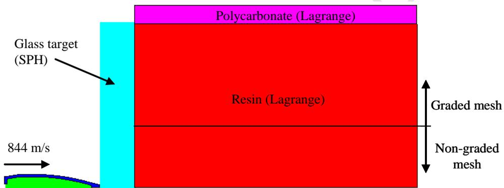
Figure 2: Numerical model set-up.
