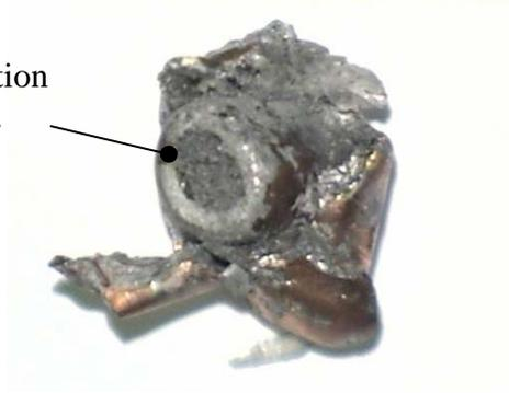
**Figure 11: Recovered bullet after completely penetrating a 6-mm glass-faced PRR target (beer-cup surround).**
