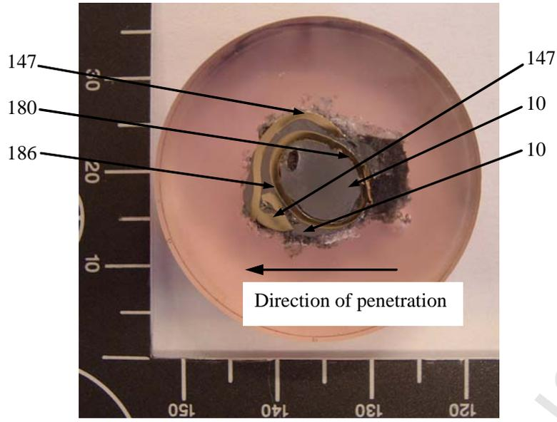
**Figure 6: Vickers microhardness (100gF load) measurements of the gilding jacket and lead antimony at the head of the bullet remains after it has completely penetrated 6 mm of glass and penetrated the PRR (polycarbonate surround).**
