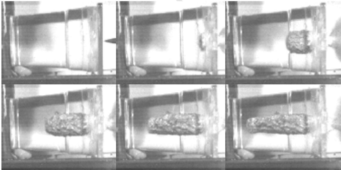
**Figure 7: Penetration of a 7.62 mm x 51 mm NATO Ball round into a 6-mm glass-faced PRR target (beer-cup surround); time between frames = 50  $\mu$ s. The curved surfaces of the beer-cup produce a lens effect and consequently the penetrating mass appears larger in diameter than it actually is.**
