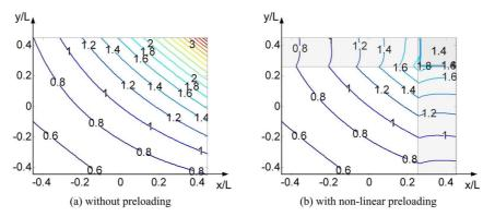
**Fig. 5** Compliance maps for cases of: (a) manipulator without preloading; (b) manipulator with preloading non-linear springs with  $K_{\vartheta} = 0.5~K_{\theta}~L^2$  and  $\vartheta_0 = \pi/12$  (b).
