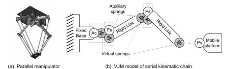
Fig. 1 Typical parallel manipulator and VJM-model of its kinematic chain.
