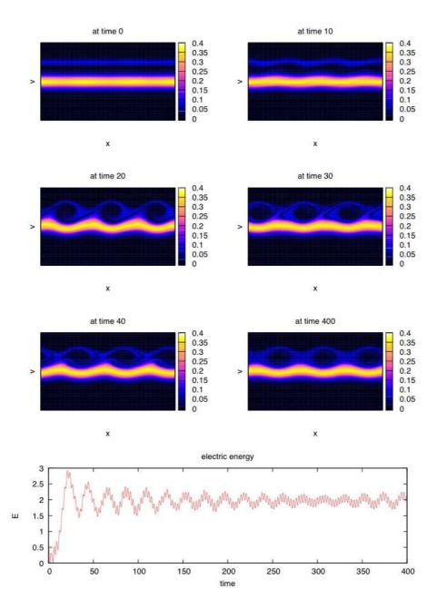
Figure 8: **Bump-On-Tail.** The evolution of the distribution functions for the Bump-On-Tail, and of the electric energy. Here d=5,  $N_x \times N_v=30 \times 30$ , the time step  $\Delta t$  is chosen by the method itself in order to limit the displacement to one cell.
