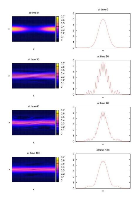
Figure 5: **Strong Landau damping.** The evolution of the distribution function and the velocity distribution for the nonlinear Landau damping. Here d=4,  $N_x\times N_v=30\times 30$ , the time step  $\Delta t$  is chosen by the method itself in order to limit the displacement to one cell.
