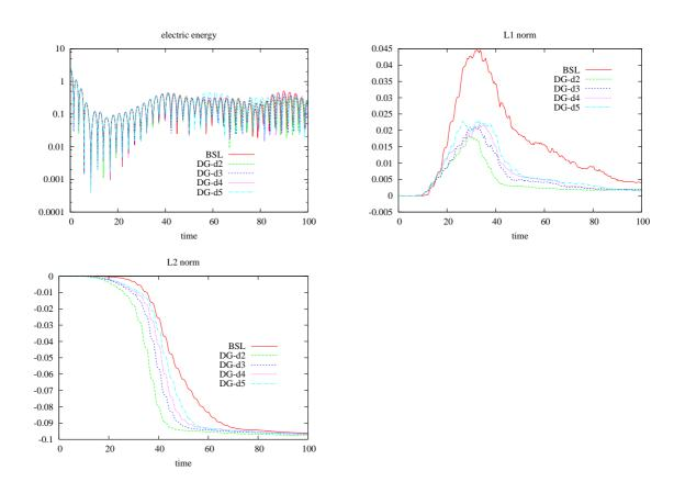
Figure 6: **Strong Landau damping.** The time evolution of the scalar magnitudes for the strong Landau damping test with a cubic splines reconstruction and DG method. Here  $N_x = N_v = 150$  for BSL and  $d, N_x = N_v$  such that  $(d+1) \times N_x = (d+1) \times N_v$  is nearly fixed to 150 for DG (d=2,3,4,5). The time step is  $\Delta t = 0.1$  for both methods. Left: electric energy (log scale); middle:  $L^1$ -norm; right:  $L^2$ -norm.
