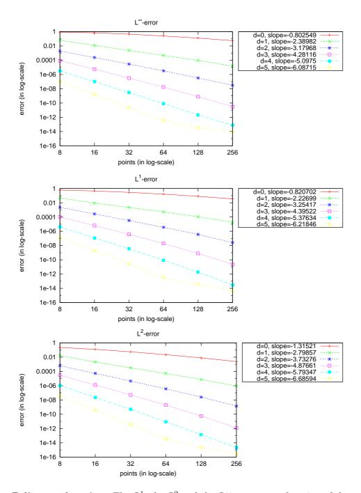
Figure 3: **1D linear advection.** The  $L^1$ , the  $L^2$  and the  $L^\infty$  errors as a function of the number of points, committed with respect to the exact solution, for the initial function  $f^0(x) = \sin(2\pi x - \pi)$ , in the interval [0,1] with periodic boundary conditions.
