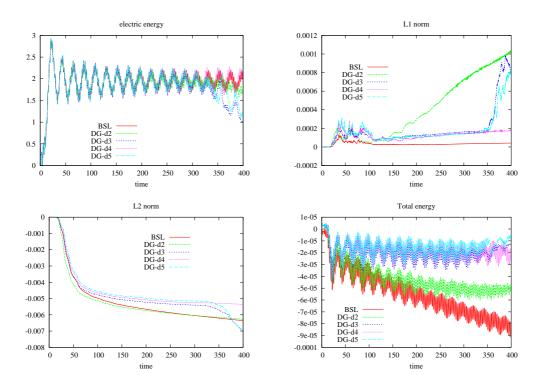
Figure 9: **Bump-On-Tail.** The time evolution of the scalar magnitudes for the Bump-On-Tail with a BSL and DG method. Here  $N_x = N_v = 150$  for BSL and  $(d+1) \times N_x = (d+1) \times N_v$  is kept nearly constant equal to 150:  $d=2, N_x=N_v=50$ ;  $d=3, N_x=N_v=38$ ;  $d=4, N_x=N_v=30$ ;  $d=5, N_x=N_v=25$ . The time step is  $\Delta t=0.1$  for both methods. Top left: electric energy; top right:  $L^1$ -norm; bottom left:  $L^2$ -norm; bottom right: total energy.
