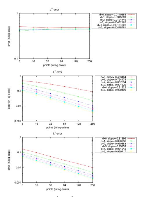
Figure 4: **1D linear advection.** The  $L^1$ , the  $L^2$  and the  $L^\infty$  errors as a function of the number of points, committed with respect to the exact solution, for the initial function  $f^0(x) = \chi_{[0,\frac{1}{2}]}(x)$ , in the interval [0,1] with periodic boundary conditions.
