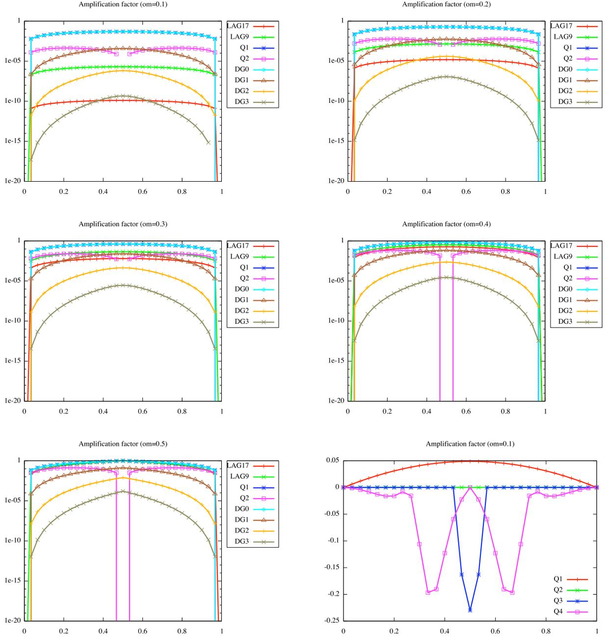
Figure 2: **Amplification factor:**  $(1 - \rho(\omega))$  is plotted for different values of  $\omega$  ( $\omega = 0.1, 0.2, 0.3, 0.4, 0.5$  and again  $0.1$ ) and different schemes, as a function of the normalized displacement  $\alpha \in [0, 1]$ .
