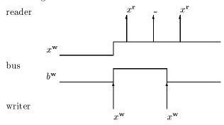
Flag switches are detected by the reader by a non predictable but bounded delay according to *physical* time: perfect physical synchrony is lost.
