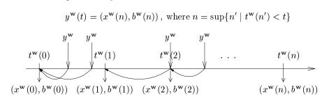
Bus. At  $t^{\mathbf{b}}(n)$ , the bus bus fetches  $y^{\mathbf{w}}$  to store in the input buffer of the reader, denoted by  $y^{\mathbf{b}}$ . Thus, at any time t, the reader input buffer is defined by:
