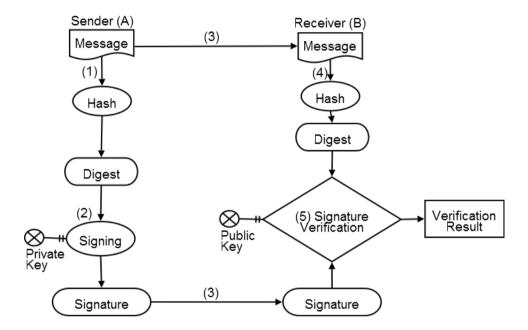
Fig. 17.6 Assuring non-repudiation using Digital Signatures
