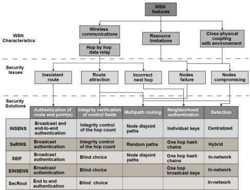
Fig. 17.8 Taxonomy of Secure Route Construction in WSN
