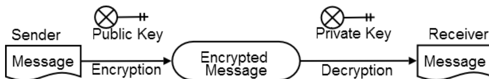
Fig. 17.5 Assuring confidentiality using asymmetric-key encryption
