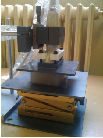
Figure 1: Measurement setup. The ultrasonic probe and a compressor plate attached to it along with an actuator were held perpendicular to the phantom by a support.
