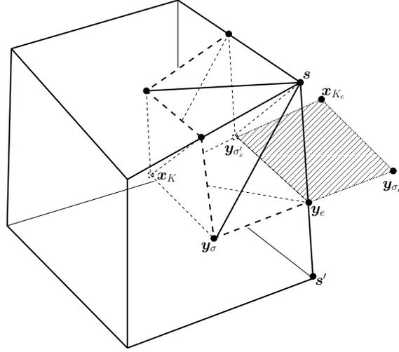
Figure 4: Construction of the submesh  $M_{K,s}$  of a control volume
