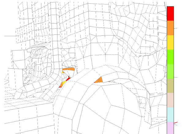
Figure 14 Intensity emitted by the engine (20 dB dynamic range, 2 dB per colour)
