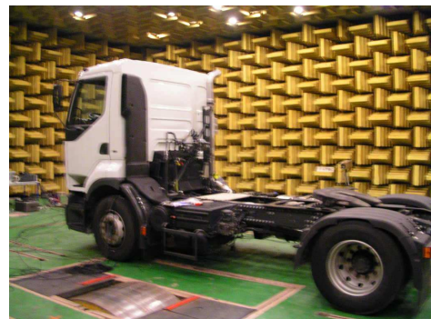
Figure 10 Transfer function measurement on truck
