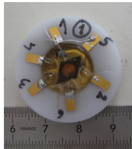
Figure 4: Photo of the whole probe after backing filling and electrical connection for characterization tests (the back side is grounded)
