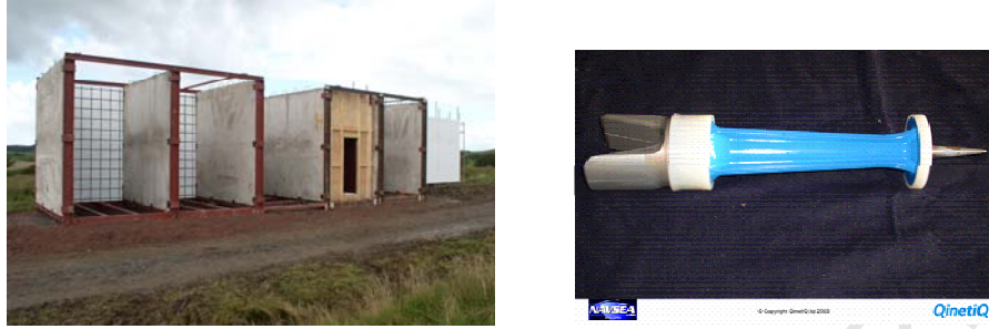
Fig. 4. Representative Target (left), projectile fired out of QinetiQ EM Gun
