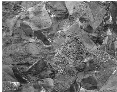
(b) cold worked (cold expanded), grains showing glide bands
