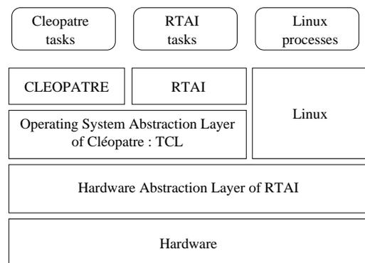
Figure 3 Software layers using Cléopatre, with RTAI.
