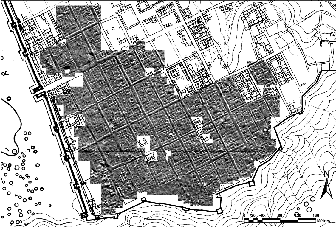
Figure 3. Magnetic map of the southern part of the city (scale -5/+5 nT/m).
