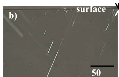
Fig. 1: a) 30 mm diameter 3C-SiC thick layer nearly free of DPB. Cross-polarized optical microscopy in the high DPB density area. DPBs are observed b) in cross-section and c) in planar view geometries.
