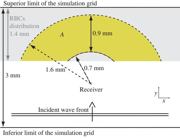
FIGURE 1 – Sketch of the computational domain. The area of interest  $A$  is the zone containing the RBCs distribution and located between the two arcs of circles. The center of these circles corresponds to the receiver position and the circle radii are 0.7 mm and 1.6 mm.
