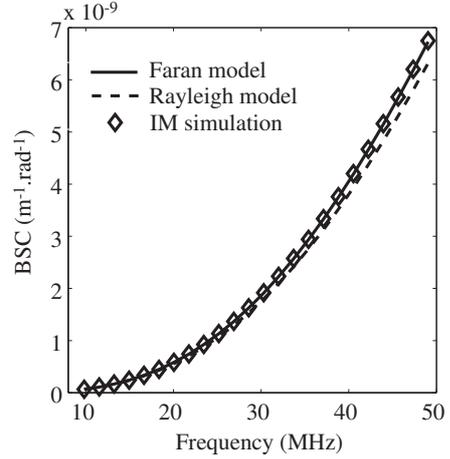
FIGURE 2 – Backscattering cross sections per unit area  $\sigma_b$  of a single RBC. The solid and dashed lines give  $\sigma_b$  given by, respectively, the Faran and Rayleigh models. Simulations results are shown by the symbols.
