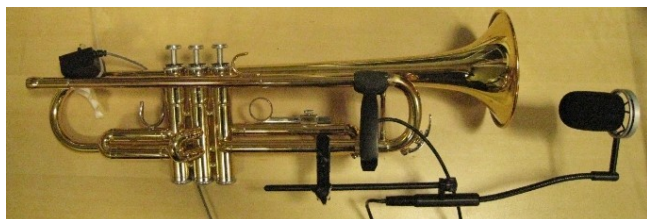
Figure 2: Bb Yamaha trumpet used for experiments. Pressure transducer, tachometer and studio microphone are fixed on the instrument.
