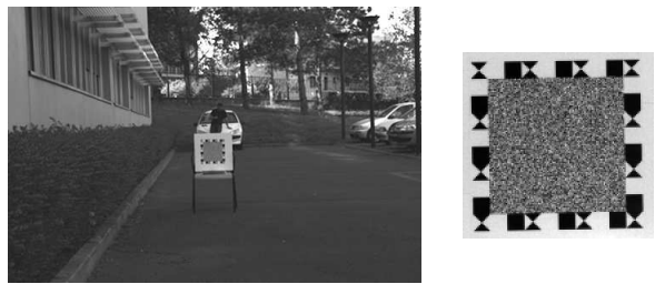
Fig. 10: Real camera example . Taken at f/5.7 . An example image, to show how local the PSF estimation is (left), and a zoom of the observed window of size 110 \times 110 pixels (right).
