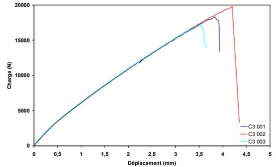
d) Matériau C3 : [(0<sub>2</sub>/90<sub>2</sub>)]<sub>s</sub>
