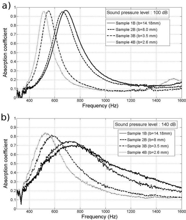
FIG. 7 – Experimental results of the absorption coefficient of the samples of group B as a function of the frequency. for a) 100 dB; b) 140 dB. Focus on the distribution effect.
