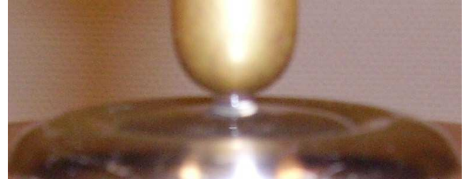
Figure 7. Motion of the water/air interface with the rod electrode.
