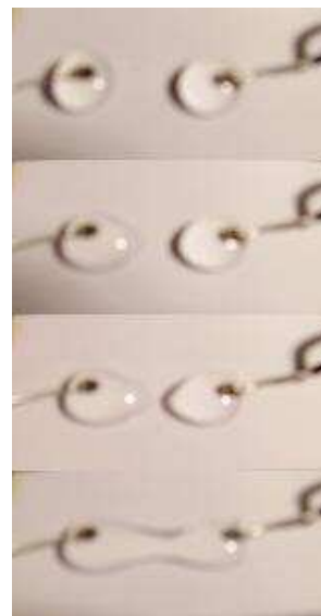
Figure 12. Deformation of a pair of electrified water drops.
