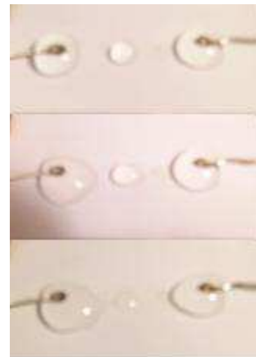
Figure 14. Deformation of a pair of electrified water drops with inserted third drop.
