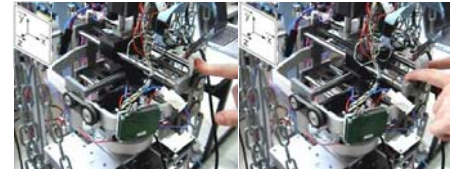
Fig.12. External forces are applied manually during successive short moments following the X direction here (left: pushing; right pulling).
