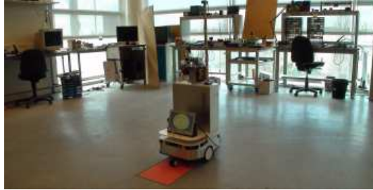
Fig. 1. The experimental set-up. The environment is a 6m x 8m area. The robot is a Robulab 10 from Robosoft with a 360 degree pan camera and a magnetic compass.
