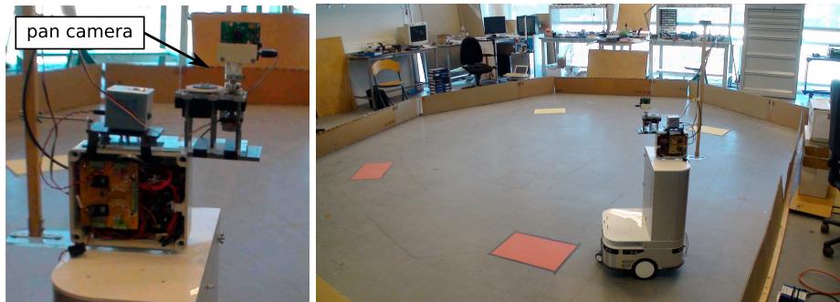
Fig. 1. The robot in its environment (equipped with a color detector placed under it). Colored squares on the ground are simulated resources.
