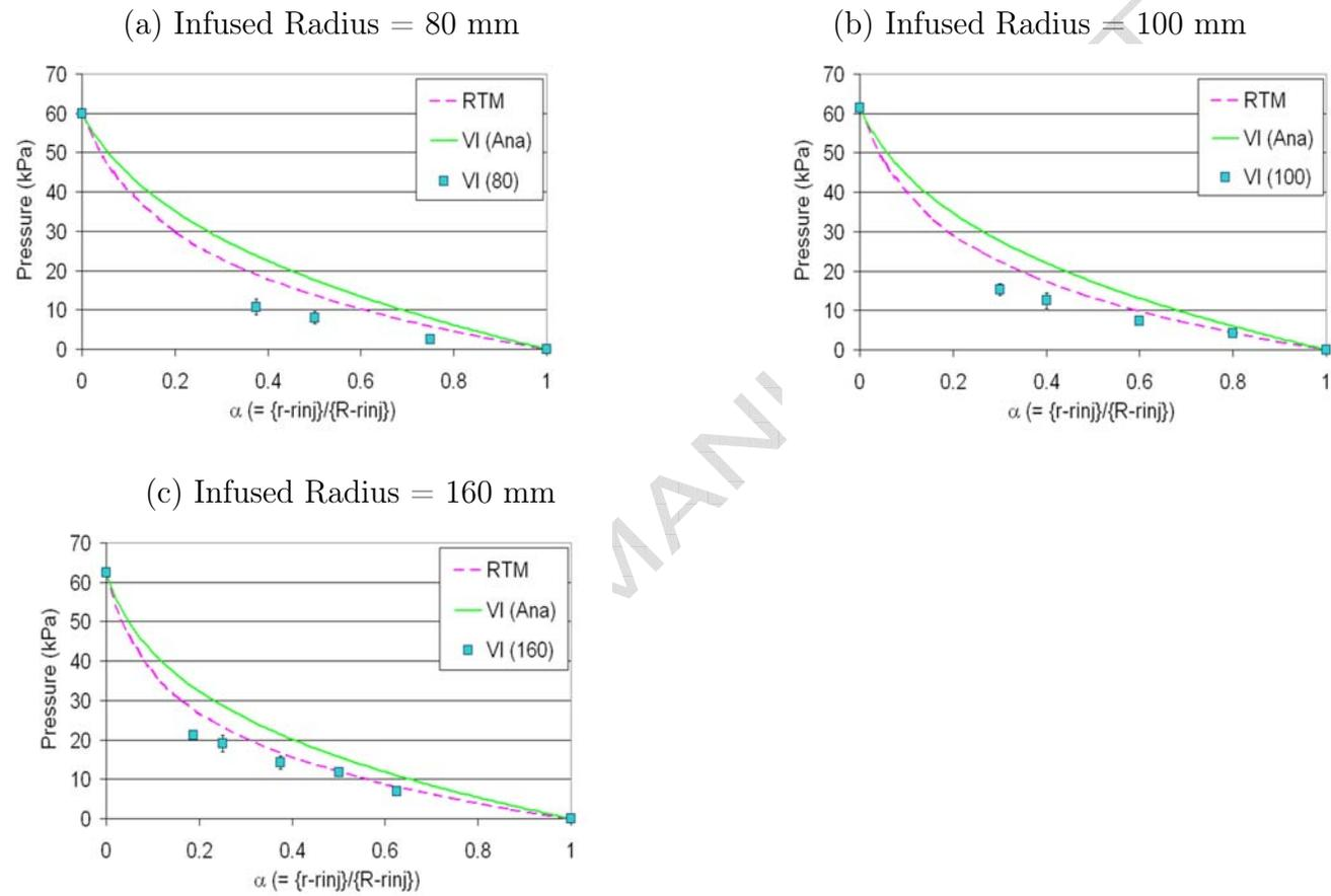
Figure 5. Pressure profile evolution with flow progression in the radial flow VI experiments.
