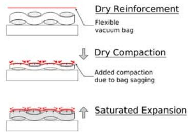
Figure 6. Comparison of events in the reinforcement compliance experiment and the actual VI process.
