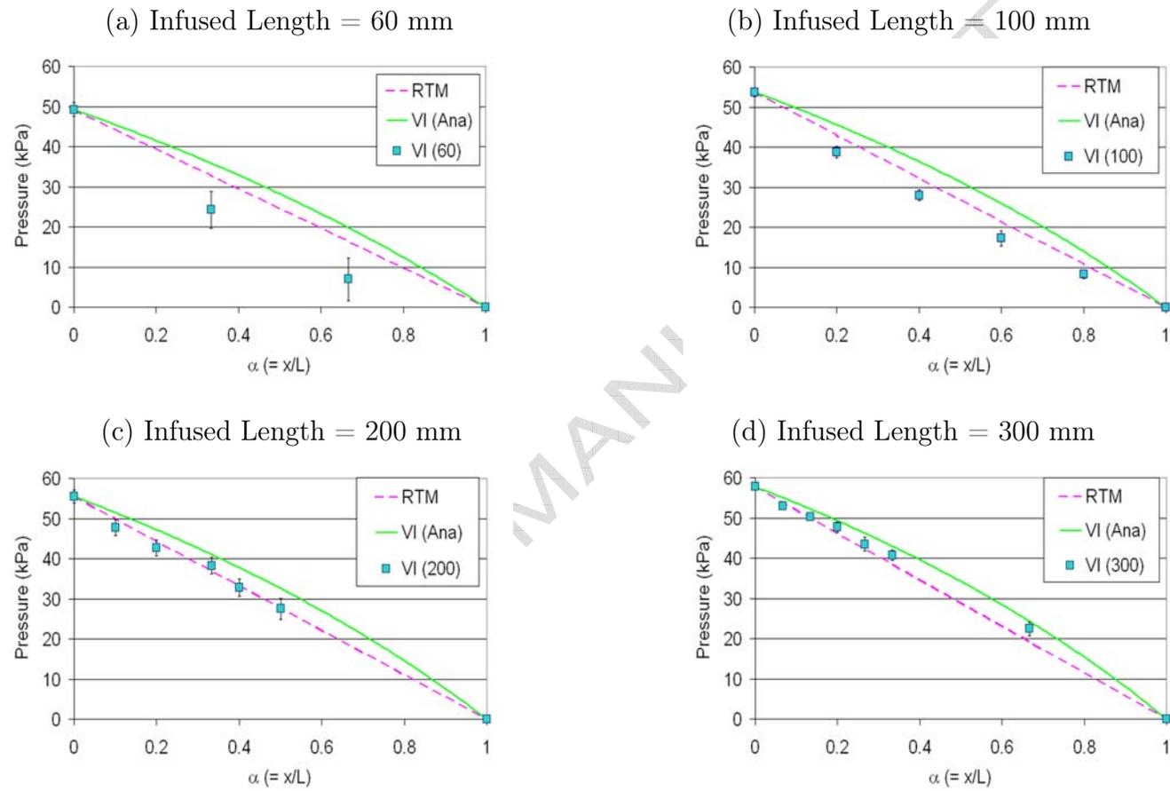
Figure 4. Pressure profile evolution with flow progression in the rectilinear flow VI experiments.
