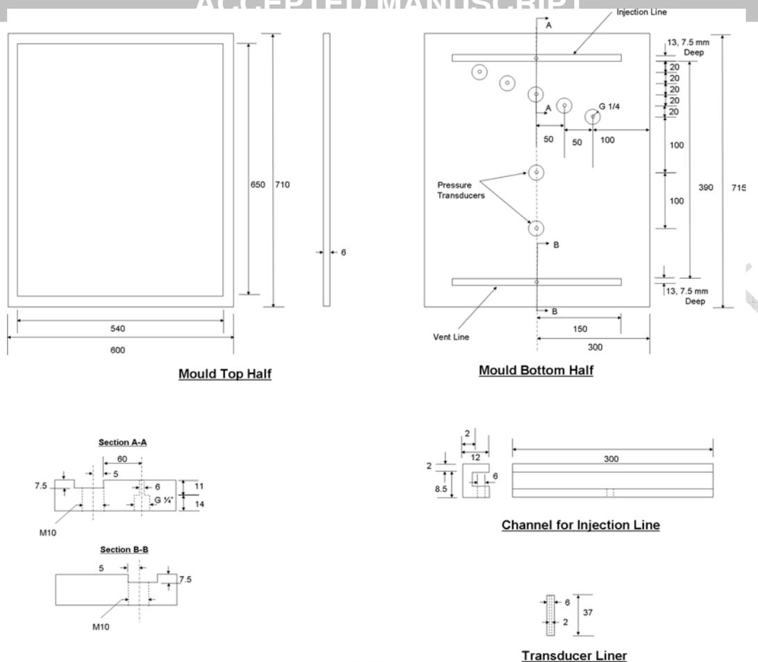
Figure 1. Experimental set-up for the rectilinear (1D) flow VI process. More pressure transducers are accommodated in this set-up by placing them across the width of the mould.
