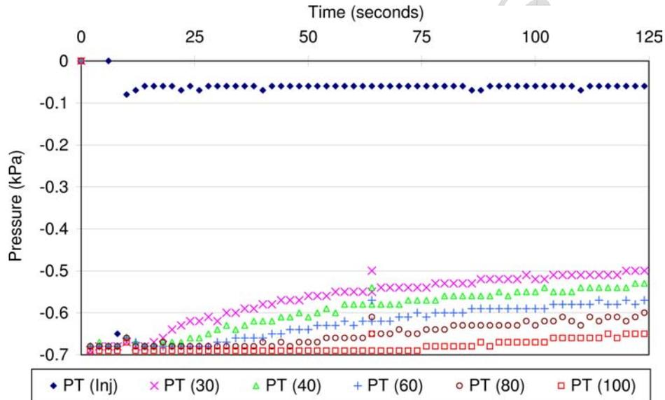
Figure 3. Pressure measurements in the rectilinear and the radial flow VI processes. The location of any pressure transducer (PT) from the injection gate is signified by the number in bracket, e.g. PT(20) = pressure transducer located at 20 mm from the injection gate.
