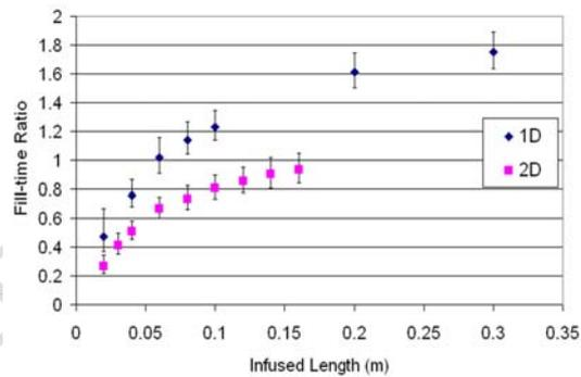
Figure 7. RTM vs. VI fill-times ratios calculated as a function of flow progression in the rectilinear and the radial flow processes.
