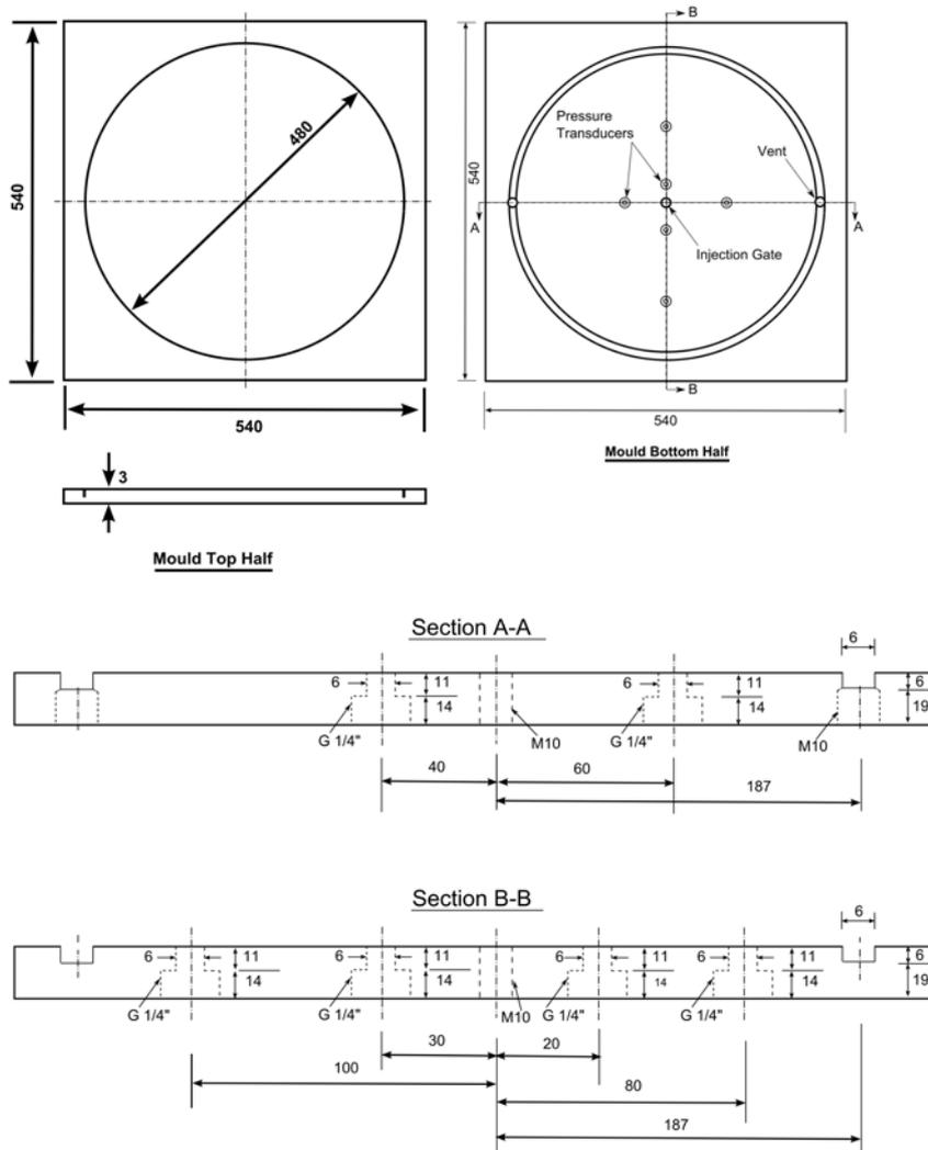
Figure 2. Experimental set-up for the radial flow VI process.
