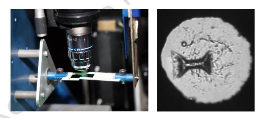
Figure 2 : Detail of the experimental setting for Raman examination of the single filament fibre under controlled load; the PET fibre in the diamond-anvil cell (cell diameter  $\sim 200 \mu m$ ).
