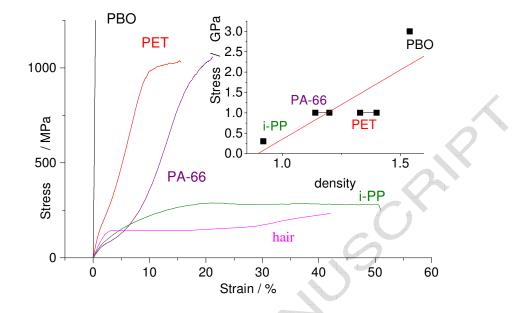
Figure 1 : Stress-strain plots for studied fibres (note the PBO stress reaches  $\sim$ 3 GPa) and the correlation between ultimate strength and density.
