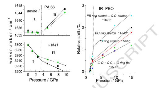
**Figure 7** : Example of Raman and IR wavenumber shift as a function of hydrostatic pressure for the PA 66 and PBO single fibre for different probes. Note the PA 66 macromolecule accommodates the pressure below 4 GPa.
