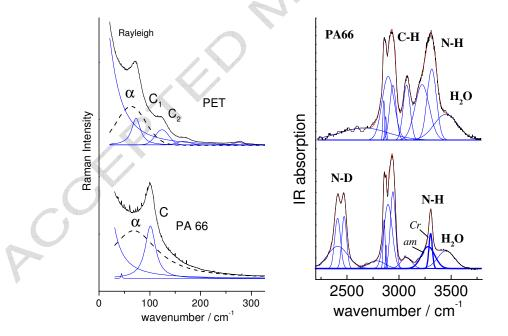
**Figure 4** : Collective low wavenumber Raman modes in // polarisation for PET and PA 66 single fibres. Comparison between IR signatures of pristine and deuterated (H isotopically diluted) PA 66 single fibre. Broad and narrow components respectively show the amorphous ( $\alpha$ ,am) and crystalline (C,Cr) conformations.
