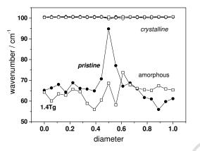
**Figure 5** : Plot of the crystalline and amorphous low wavenumber component across the diameter ( $\sim 30\mu m$ ) of a PA 66 single fibre, before and after heating above the Tg temperature.
