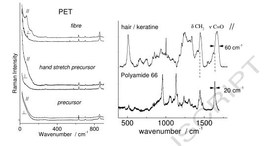
**Figure 3** : Examples of polarised Raman spectra showing the (PET) crystallisation and texturation of a amorphous precursor filament under tension into a high crystalline oriented fibre; comparison between polarised spectra of high crystalline polyamide and low crystalline keratin fibres.
