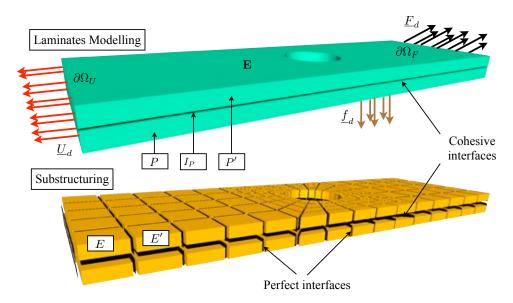
Figure 6: Substructuring of the laminated composite structure
