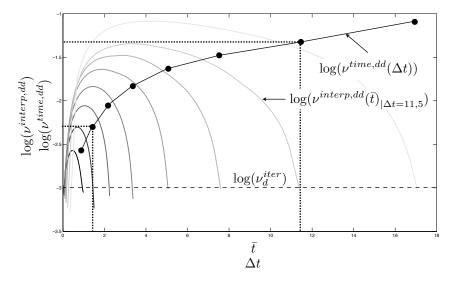
Figure 10: Grey curves: evolution of  $\nu^{interp,dd}$  as a function of  $\bar{t} \in [t_n \ t_{n+1}]$  for different values of  $\Delta t$ . Black curve: Evolution of  $\nu^{time,dd}$  with respect to  $\Delta t$  (maximum values of the gray curves)
