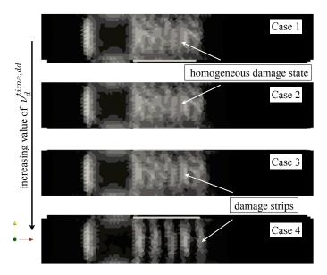
Figure 3: Influence of the prescribed value  $\nu_d^{time,dd}$  on the damage state in the upper cohesive interface of the DCB problem
