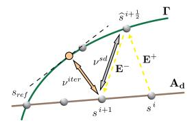
Figure 9: Classical convergence indicator  $\nu^{sd}$  of the LaTIn solver and indicator  $\nu^{iter}$  based on the error in the constitutive law
