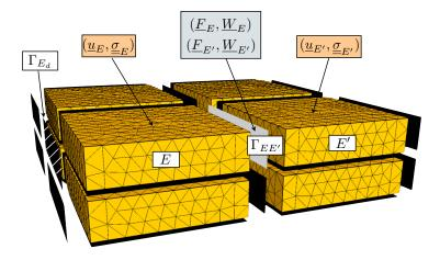
Figure 7: Substructuring of the laminated composite structure
