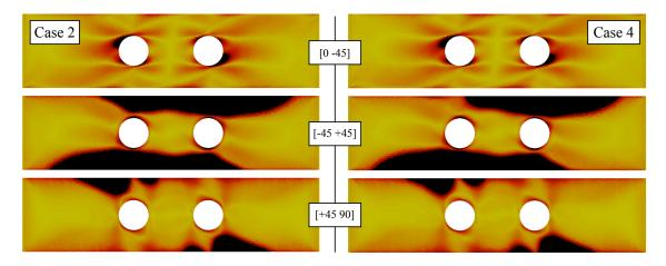
Figure 17: Damage state in the interfaces of the holed plate at the beginning of an instability obtained in a converged case (prescribed arc-length, Case 2), and by using the time control procedure (fixed discretization error, Case 4)
