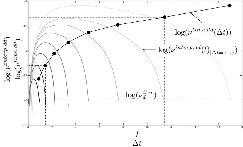
Figure 10: Grey curves : evolution of  $\nu^{interp,dd}$  as a function of  $\bar{t} \in [t_n t_{n+1}]$  for different values of  $\Delta t$ . Black curve: Evolution of  $\nu^{time,dd}$  with respect to  $\Delta t$  (maximum values of the gray curves)
