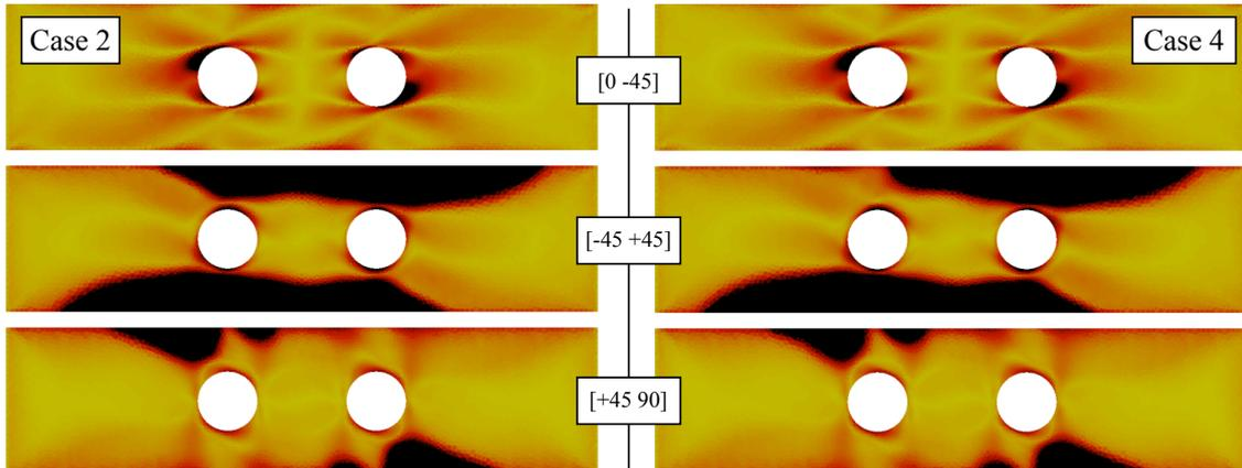
Figure 17: Damage state in the interfaces of the holed plate at the beginning of an instability obtained in a converged case (prescribed arc-length, Case 2), and by using the time control procedure (fixed discretization error, Case 4)
