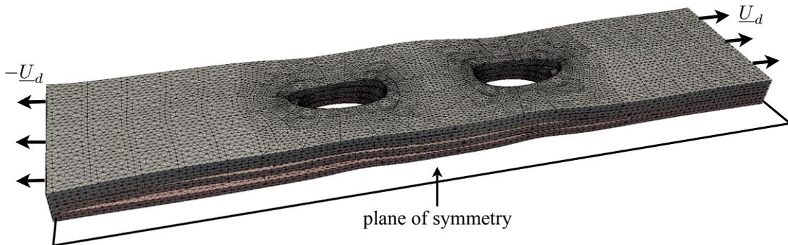
Figure 12: Definition of the holed plate problem (317 000 d.o.f.)
