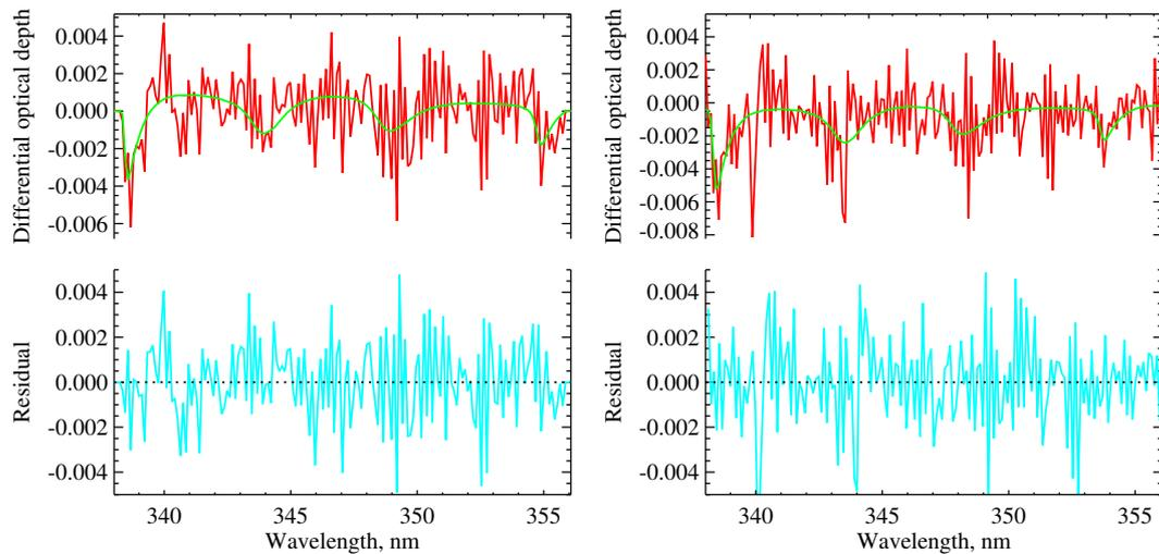
**Fig. 4.** Example spectral fits at a tangent height of 21 km for IUP Bremen (left panels) and MPI Mainz (right panels) algorithms. Upper panels show measured (red) and simulated (green) optical depths of BrO while lower panels show fit residuals.
