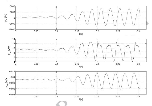
Figure 10 – Time history of a) static pressure at the burner end of the combustion chamber (relative to atmospheric pressure), b) instantaneous thermal power released within the combustion chamber and c) fuel mass flow rate through the main radial holes during the transient CFD simulation.
