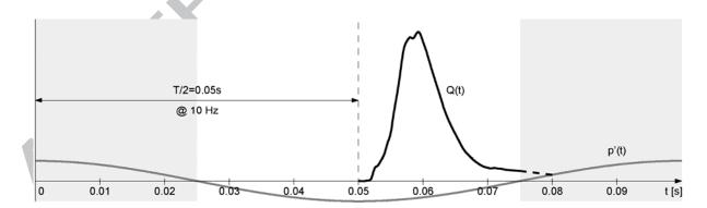
Figure 9 – Timing of the pressure fluctuation due to the acoustic mode at 10Hz and of the heat released by the fuel injected through the main radial holes (if the heat is released outside the gray zones, the necessary condition stated by Rayleigh criterion is not satisfied and thermoacoustic oscillations at this frequency are certainly dampened).
