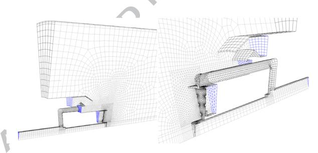
Figure 6 – Details of the unstructured grid of the reduced domain used in the stationary and transient reacting flow simulations (about 50,000 cells).
