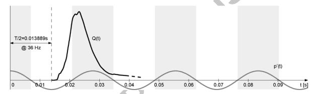
Figure 8 – Timing of the pressure fluctuation due to the acoustic mode at 36Hz and of the heat released by the fuel injected through the main radial holes (if the heat is released in the gray zones, the necessary condition stated by Rayleigh criterion is satisfied and thermoacoustic oscillations at this frequency are likely to grow).
