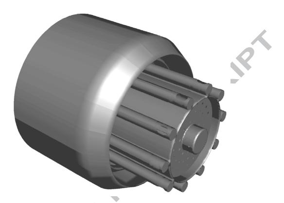
Figure 1 – The burner of the 10MW industrial boiler used as example of application.
