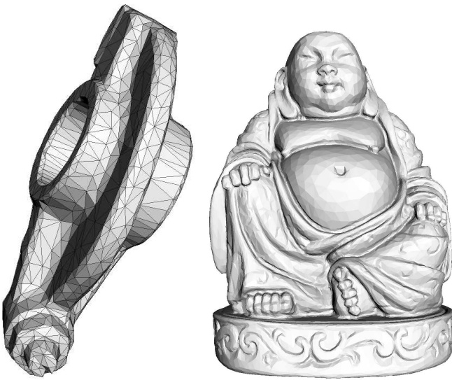
Fig. 12. Coarsened versions of the rockerarm model (1000 vertices) and the buddha model (20k vertices).
