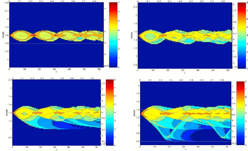
Figure 6: Velocity distribution function of particles along the  $x$  axis, when injected at  $v_b = 1.6$  (upper left),  $v_b = 1.5$  (upper right),  $v_b = 1.4$  (lower left) and  $v_b = 1.3$  (lower right), above the wave phase velocity,  $v_\phi = 1$ , with  $m = k = 1$  and wave amplitude  $A = 0.04$ . White lines mark the cat's eye boundaries  $v_\phi + 2\sqrt{A} = 1.4$  and  $v_\phi - 2\sqrt{A} = 0.6$ .
