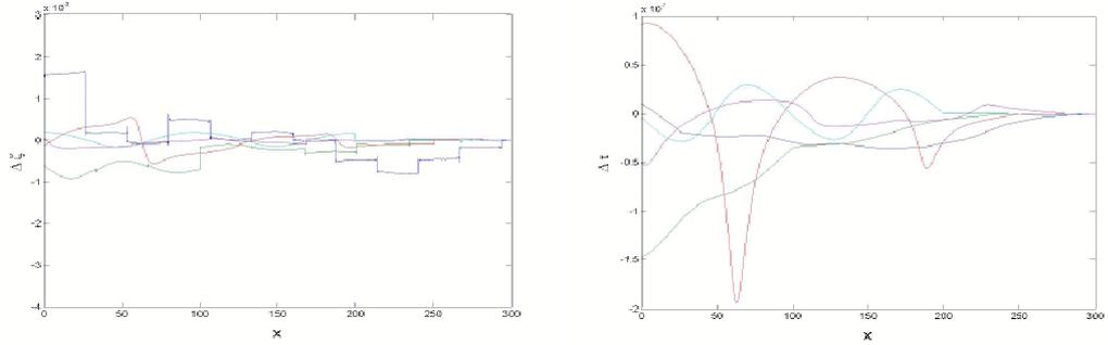
Figure 2: Discrepancy, between direct evolution  $\mathcal{F}_{\Delta x}$  and backward evolution  $\mathcal{F}_{-\Delta x}^*$ , for energy and arrival time as functions of position, for five particles in the field of a single wave with  $A = 0.1$ ,  $k = 0.2$ ,  $v_\phi = 1$ ,  $\phi = \pi$ . Particles injected at the origin at  $t = 0$  with velocities 0.6, 1.1, 1.5, 2 and 2.5.
