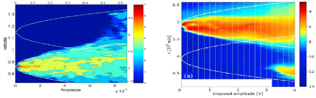
Figure 9: Velocities of particles after interaction with two waves, versus amplitude of waves  $A_1 = A_2$ . Cold beam injected at phase velocity of one wave. (left) Numerical results for  $v_b = v_{\phi_1} = 1.1487$ ,  $v_{\phi_2} = 0.8609$ ,  $k_1 = 0.6529$ ,  $k_2 = 1.7424$ . (right) Experimental data.
