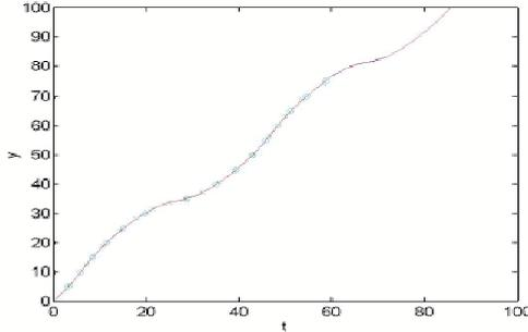
Figure 1: Sketch of the algorithm principle in  $(x, t)$  plot. The continued line is a trajectory. Crosses are positions, obtained by leap-frog with constant time step, circles mark times obtained by our approach with constant space step.
