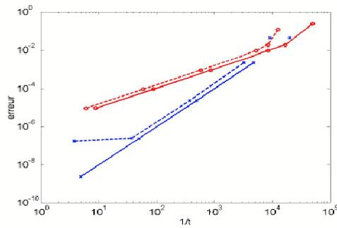
Figure 3: Numerical accuracy for the first order algorithm (red, upper lines) and second order (blue, lower lines) versus calculation time per spatial unit length. Continued line for the Newton method solution to the cubic equation, dashed line for Matlab built-in polynomial solver.
