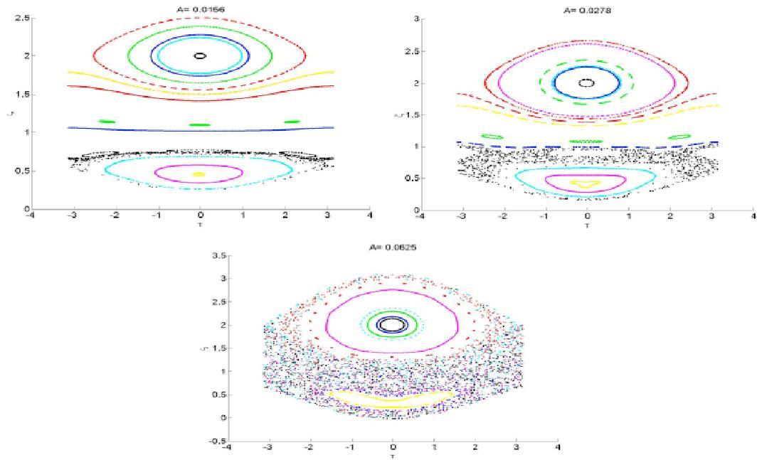
Figure 7: Poincaré section in  $(\tau, \zeta)$  variables, of the return map after one wavelength  $L$ , for 15 particles, with mass  $m = 1$ . Wave parameters are  $k_1 = 1$ ,  $k_2 = 1/2$ ,  $v_{\phi_1} = 1$ ,  $v_{\phi_2} = 2$ ,  $\phi_1 = \phi_2 = \pi$ . Wave amplitudes  $A_1 = A_2$  are chosen so that overlap parameter is  $s = 0.5$  (top left),  $0.66$  (top right) and  $1$  (bottom).
