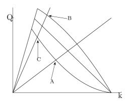
Figure 4: **Left:** Classical model. A and B fall outside of the classical fundamental diagram and are viewed as A1 and B1; the resulting steady state is B1. **Right:** Perturbed model. A and B fall in the perturbed fundamental diagram; the resulting steady state is C.
