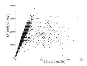
Figure 2: Experimental flow-density relations over a one week-period at two locations on a highway in Roma. Flow was directly measured and density was computed from the measured flow and the measured speed. In free-flow the speed is constant. The shape of the congestion phase changes for different locations.
