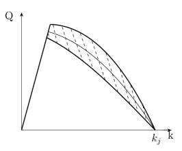
Figure 3: **Left:** Perturbed triangular fundamental diagram (the equilibrium flux function is linear decreasing in congestion). **Right:** Perturbed Greenshields fundamental diagram (the equilibrium flux function is parabolic decreasing in congestion). One can note that the free-flow speed is constant in both models and the flux is set-valued in congestion, i.e. to one density corresponds several values of the flux.
