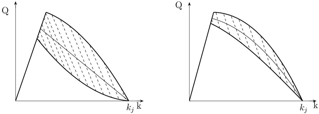
Figure 3: **Left:** Perturbed triangular fundamental diagram (the equilibrium flux function is linear decreasing in congestion). **Right:** Perturbed Greenshields fundamental diagram (the equilibrium flux function is parabolic decreasing in congestion). One can note that the free-flow speed is constant in both models and the flux is set-valued in congestion, i.e. to one density corresponds several values of the flux.
