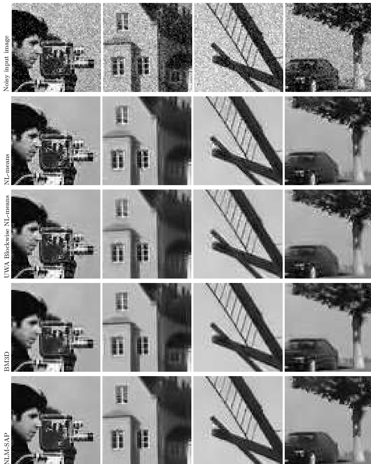
Fig. 12 Comparisons of the visual denoising performances of the proposed NLM-SAP approach and other state-of-the-art methodologies. From top to bottom, the input noisy images, the results obtained by the classical (pixelwise) NL-Means [5], the blockwise NL-Means using UWA reprojection [5], the BM3D denoiser [7], and our proposed NLM-SAP approach.
