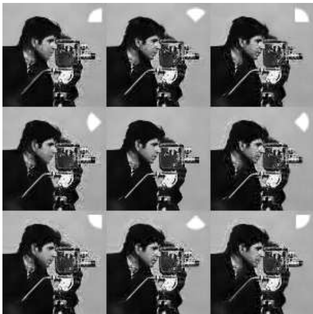
Fig. 8 Eight denoised images obtained for different oriented patch shapes. The proposed final aggregate is in the center. Each denoiser provides good performances in a specific target direction but suffers from noise halos in the other directions. The final (central) aggregate takes advantage of every oriented-denoiser to provide high quality restored edges. The patch shape used is indicated in white.
