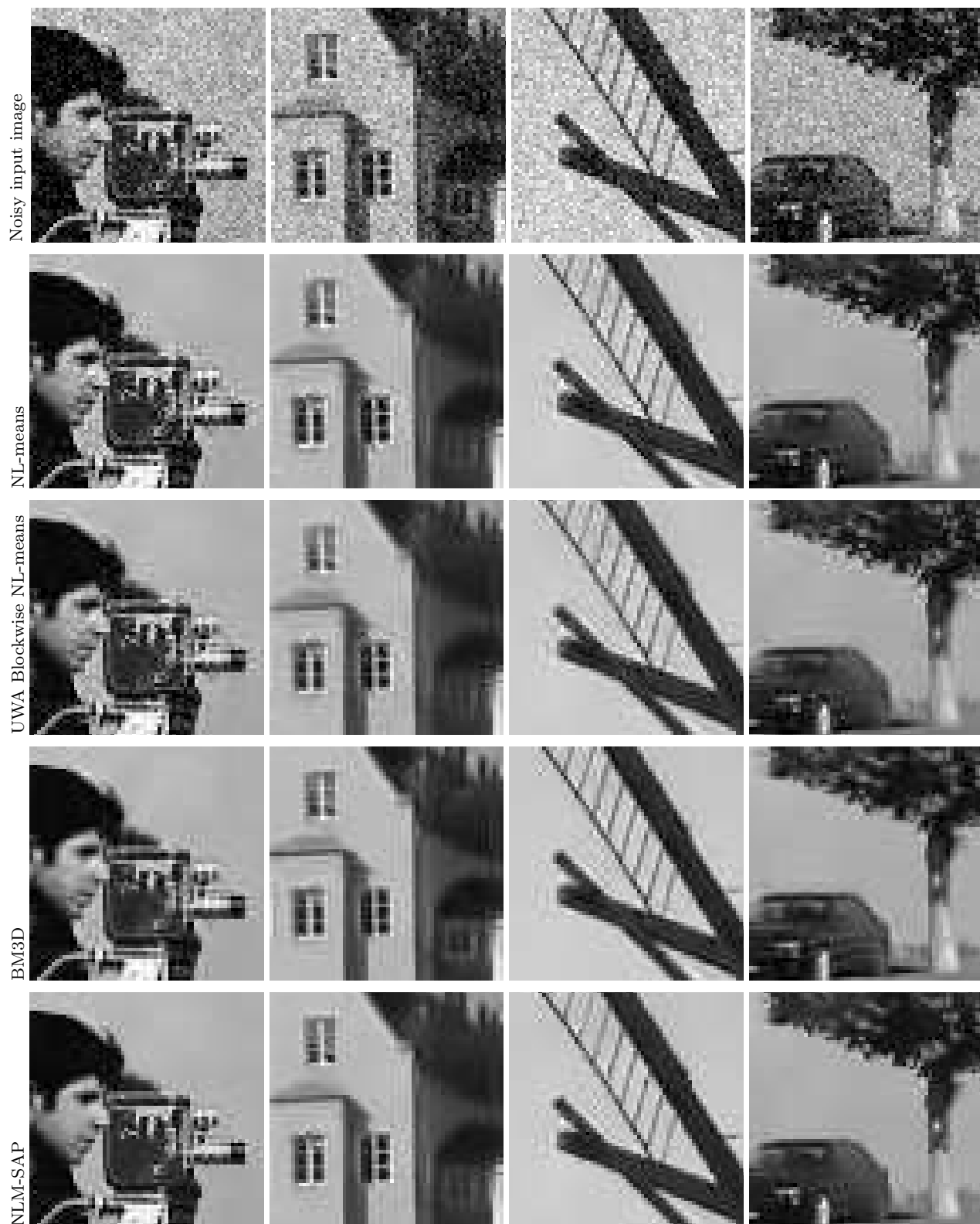
Fig. 12 Comparisons of the visual denoising performances of the proposed NLM-SAP approach and other state-of-the-art methodologies. From top to bottom, the input noisy images, the results obtained by the classical (pixelwise) NL-Means [5], the blockwise NL-Means using UWA reprojection [5], the BM3D denoiser [7], and our proposed NLM-SAP approach.
