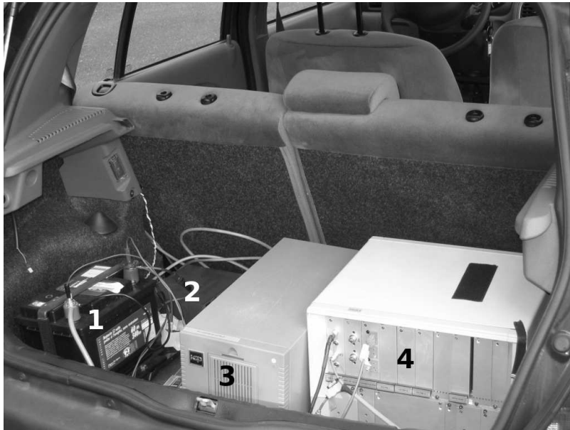
Fig. 7.3. View of the rapid prototyping system placed in the booth. 1 Lead-acid battery powering the IBM TM compatible PC and the interface rack - 2 General switch - 3 IBM TM compatible PC - 4 interface rack
