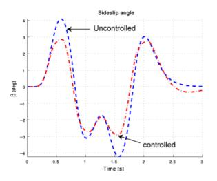
Fig.7 Sideslip angles of the controlled and uncontrolled vehicles
