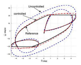
Fig. 5 Response of the yaw rate versus steering angle
