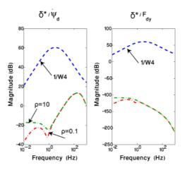
d) Closed loop transfer function between exogenous inputs and  $\delta^*$
