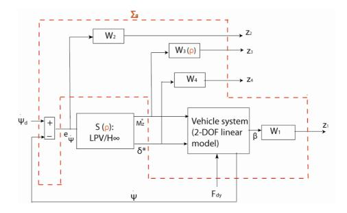
Fig.3 Generalized plant model for synthesis
