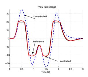
Fig.6 Yaw rate responses of the controlled and uncontrolled vehicles
