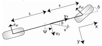
Fig.1 2-DOF model of lateral vehicle dynamics
