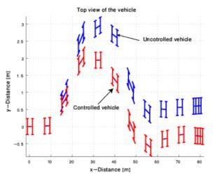
Fig.8 Trajectories of the controlled and uncontrolled vehicles
