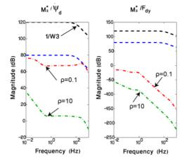
c) Closed loop transfer function between exogenous inputs and  $M_z^*$
