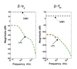
a) Closed loop transfer function between exogenous inputs and  $\beta$
